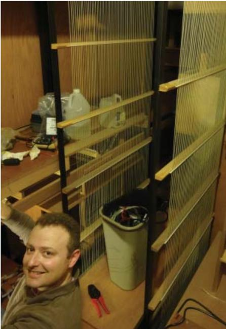
**Left:** Technician Vladimir works in the box behind the organ. The fiberglass “strings” next to him are the trackers that open the valves in the pipes when the keyboard is played.
