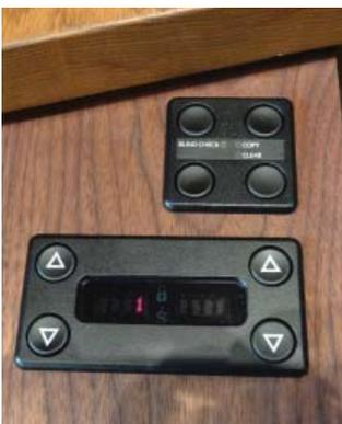
**At right:** Don DeBruin is happy with the refurbished organ. The new system handles the same 23 pistons and toe studs as before, but adds 32 memory levels, so the organ can now store 23 x 32 preset pistons. An extra toe stud cycles automatically to the next preset.
